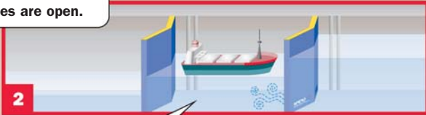
2 When all gates are shut, water is let into the lock through a sluice (small gate).
